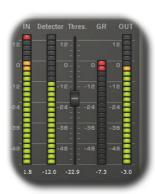
Meters for main signal (Inp), detector signal (Det), output (Out) and gain reduction (GR).
